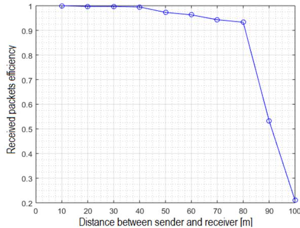
Figure 6: Packet reception rate according to the distance between OBUs
