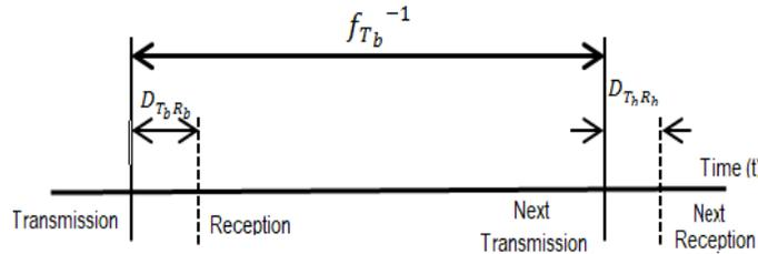
Figure 1: Key parameters to determine position error (Adapted from [4])
