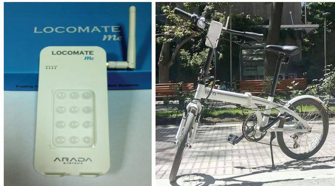
Figure 3: Arada LocomE Mobile Device and installation in the bicycle
