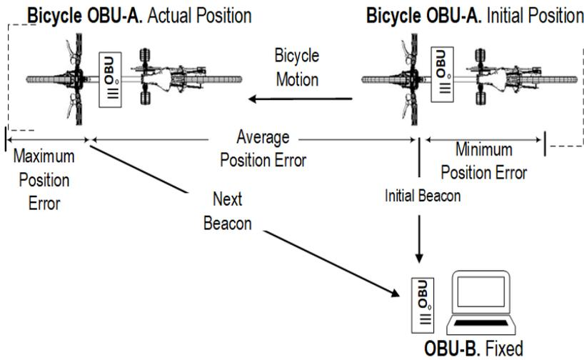
Figure 5: Schematic illustration for experimental evaluation of adaptive beaconing algorithms
