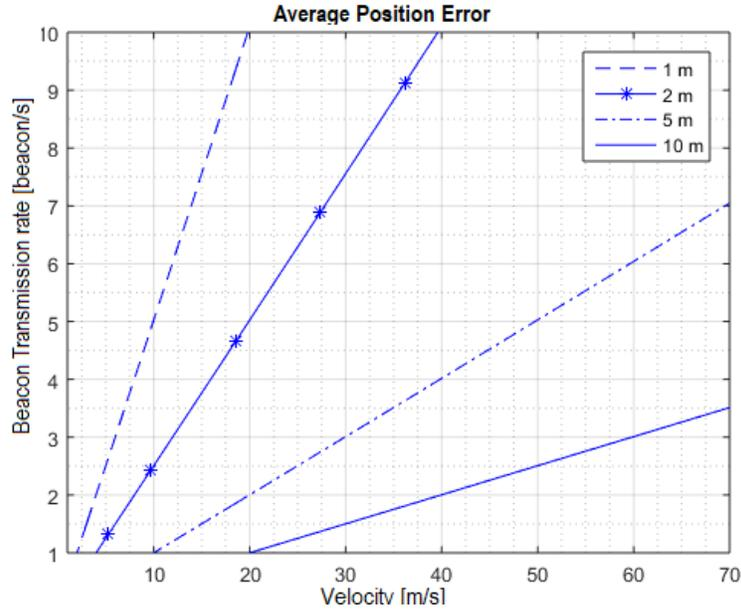
Figure 2: Average position error (m) depending on velocity and beacon transmission rate with  $D_{T_b R_b} = 0.001s$
