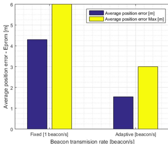
Figure 7: Average and maximum position error perceived by the fixed node
