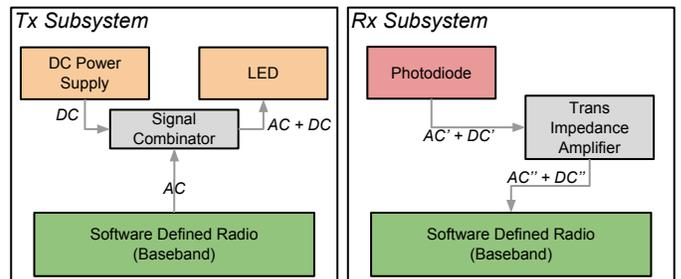
Fig. 2. Tx and Rx Subsystems of the Platform. Tx modulates the intensity of the LED and Rx detects intensity variations from the received light, converting light to electric signals. The modulation and demodulation processes are done with the SDRs.
