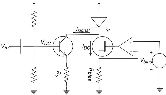
Fig. 4. Signal Combinator. It receives the DC and AC signals coming from the LED's DC power supply and the SDR output, respectively, and sends the sum of both signals to the LED. Source: [11]
