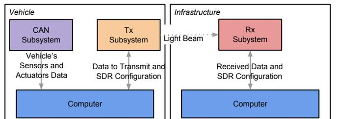
Fig. 6. V2I platform configuration.
