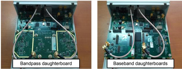
Fig. 3. Modification of the NI USRP 2922 original daughterboard (which works in bandpass) [left side] to baseband daughterboards [right side]
