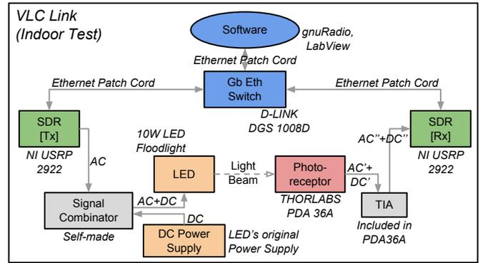
Fig. 1. Block diagram of the VLC system.
