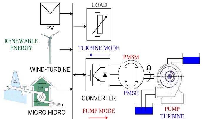
Fig. 5. Pumped storage energy storage system energized by RES [27]
