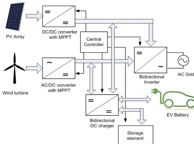
Fig. 6. RES based EV charging station diagram
