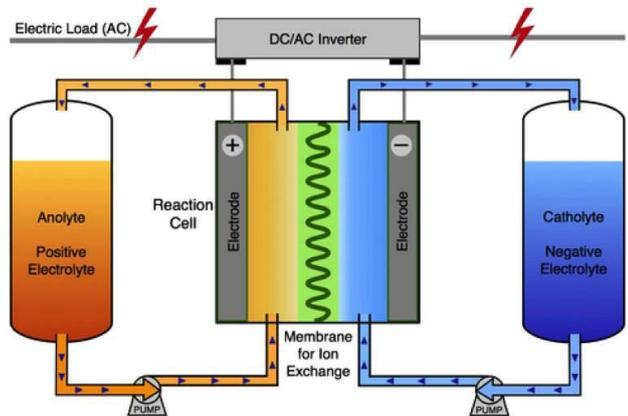
Fig. 4. The vanadium redox flow battery [29]
