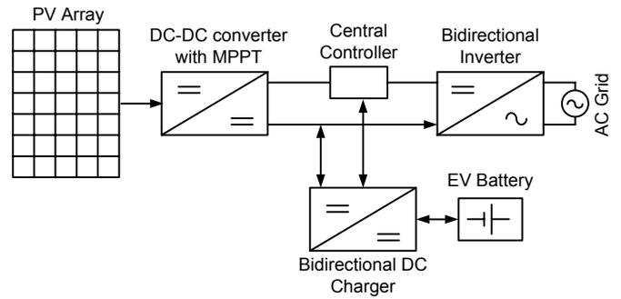
Fig.2. PV energized Charging station [16], [17]
