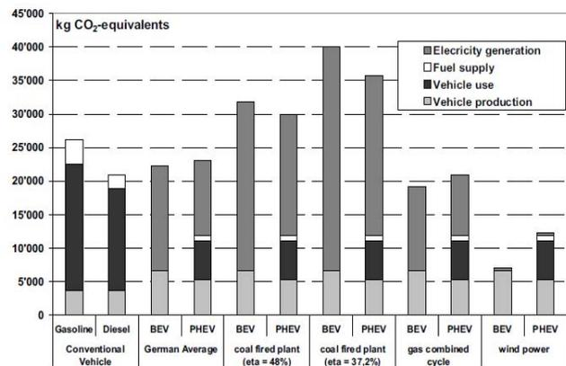
Fig. 1. CO<sub>2</sub> pollution by different types of vehicles [4]
