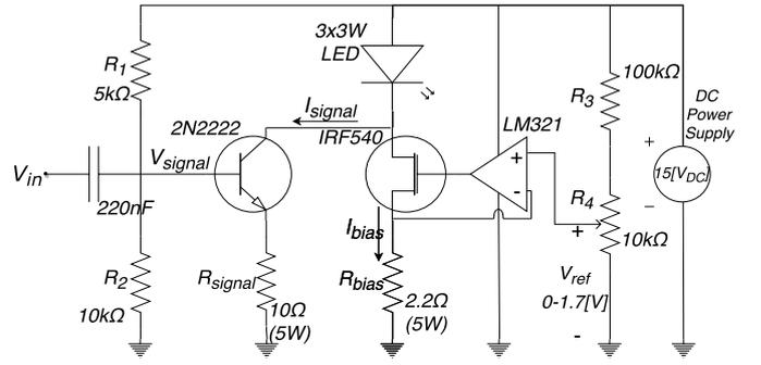
Fig. 4. Implemented Signal Combining Circuit (SCC).
