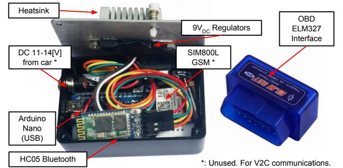
Fig. 6. CAN module implementation using Arduino Nano, HC05 Bluetooth circuit, SIM800L GSM circuit (for vehicle-to-cloud communication purposes), and an OBD interface based on ELM327 circuit.
