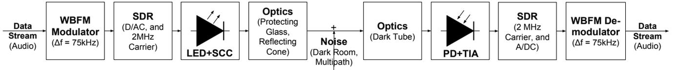
Fig. 7. Block diagram of the software developed in GNU Radio for the SDRs along with the VLC hardware implemented.
