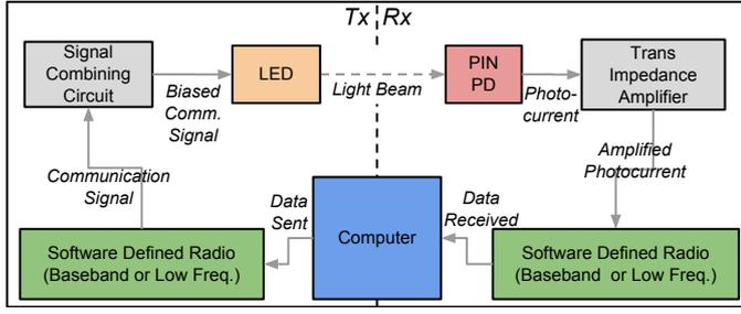
Fig. 2. VLC module blocks.
