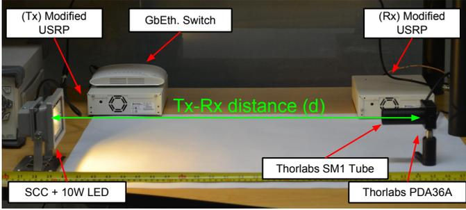
Fig. 3. A laboratory setup of the VLC module.
