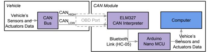
Fig. 5. CAN platform subsystem capable of reading the data of the CAN Bus.
