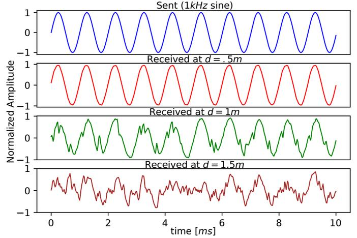
Fig. 8. Comparison of 1kHz sine communicated through the VLC module varying Tx-Rx distance  $d$ .
