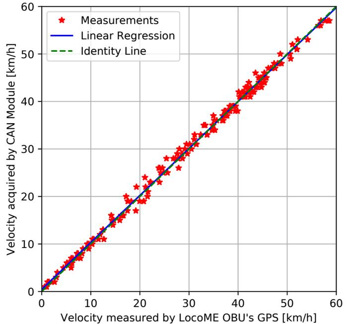
Fig. 9. Velocity data acquired with CAN module and estimated by the GPS of an Arada Systems LocoMate ME OBU.
