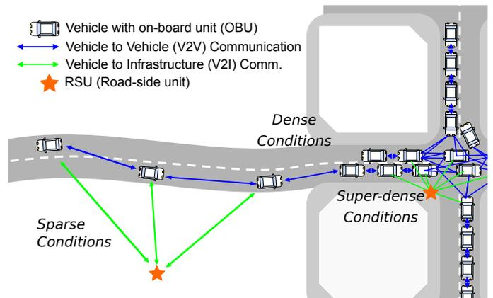
Fig. 1. Basic architecture of vehicular networks, conformed by on-board units (OBUs) inside cars, and road-side units (RSUs) hosted by the vehicular infrastructure that communicate under vehicle-to-vehicle (V2V) and vehicle-to-infrastructure (V2I) schemes.
